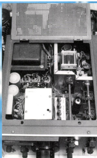
Fig. 4: Inside view of the T-599S transmitter. The p.a. stage is on the top right within the screened compartment, and the v.f.o. on the bottom left. Linking between the variable capacitor control shafts and the capacitors is by substantial 'non slip' chain drives!
